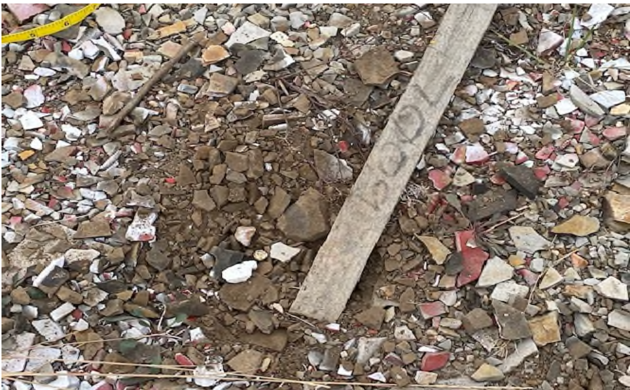
Figure 4: Installed base station control point (nail head)
