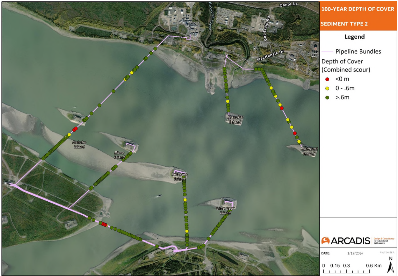
Figure 26. Minimum Depth of Cover During the 100-Year Event with the Sediment Type 2 Scenario
