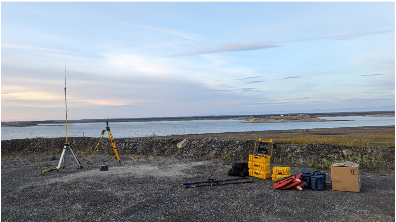
Figure 3: Base station with antennae installed during 2023 survey activities
