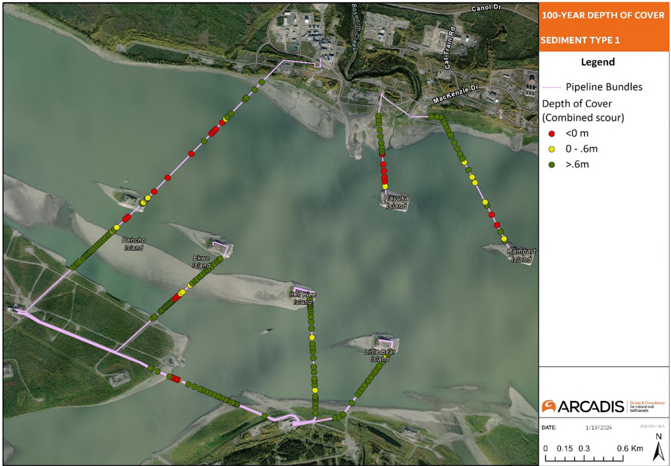
Figure 27. Minimum Depth of Cover During the 100-Year Event with the Sediment Type 1 Scenario
